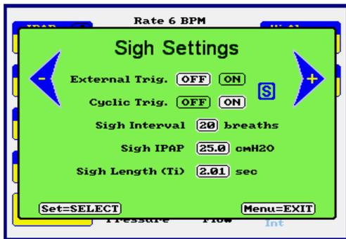
Use the SET button to scroll down the settings, using the +/- buttons to alter the settings.
