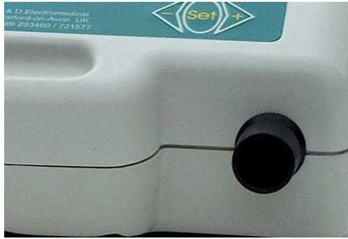
1. **Outlet** - Main Air Outlet to breathing circuit
